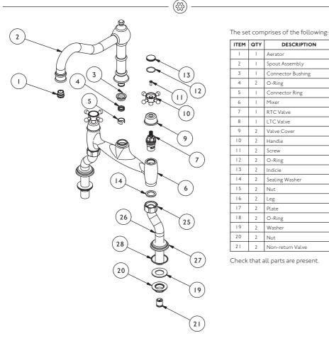
ITEM QTY DESCRIPTION 1 Aerator 2 Spout Assembly 3 Connector Bushing 4 2 O-Ring 5 Connector Ring 6 1 Mixer 7 RTC Valve LTC Valve 8 1 9 2 Valve Cover 10 2 Handle 11 2 Screw 2 O-Ring 12 13 2 Indicie |4 2 Sealing Washer 15 2 Nut 16 2 Leg 17 2 Plate 18 2 O-Ring 19 2 Washer 20 2 Nut 21
