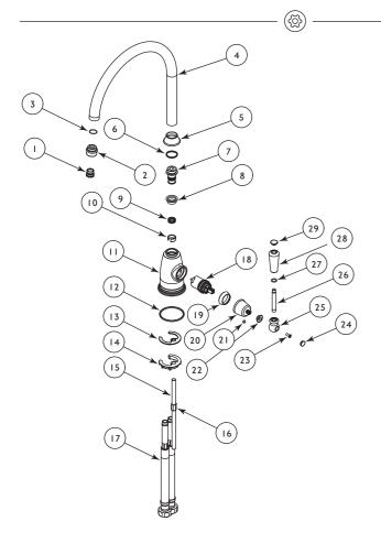
ITEM QTY DESCRIPTION Aerator 1 Aerator Housing 2 3 O-Ring 4 Spout 5 Spout Cover Spout Bushing 6 7 Connector Connector Bushing 8 Q 2 O-Ring Connector Ring 10 11 Mixer Body 12 O-Ring 13 Washer 1 14 Horseshoe Plate 15 Fixing Stud 1 16 Fixing Nut 17 MI2 x G¾" Connection 2 18 Cartridge 19 Cartridge Ring Cartridge Cover 20 21 Screw 22 Handle Ring 23 Screw 24 Indicie 1 25 Handle 26 Handle Stem 27 O-Ring 28 Ceramic Lever 29 Ceramic Handle Nut
