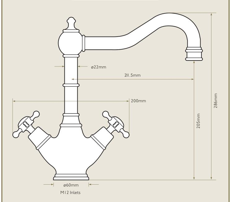
RECOMMENDED HOLE SIZE 35mm Supplied with 400mm flexi tails (G³¼" connection) ENSURE CORRECT PRESSURE BEFORE FITTING: Minimum operating pressure 0.3 Bar Recommended operating pressure 1.0 Bar Maximum operating pressure 3.0 Bar
