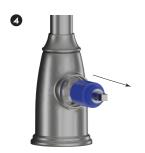
Remove the cartridge from the body of the tap
